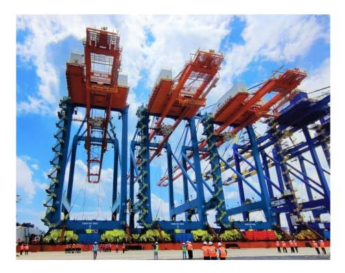
VCT received the shipment carrying 3 Quay Cranes from ZPMC on 9th Sept 2021. These Super Post Panamax Quay Cranes are equipped with the latest technology for efficient handling of containers. These cranes have an outreach to handle 22 containers across vessels and can perform twin lift container handling up to 65 tonnes under spreader.
